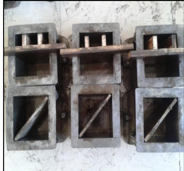
Fig. no.4: Vertical and Diagonal joints of interface layer in plan
